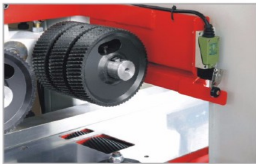
The before work table is equipped with the active feeding wheel, powerful feeding.
