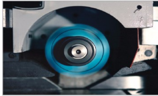
Front and rear press plate can be adjusted respectively, although the big variation in wood thickness, also work pieces can be firmly pressed down on the working table
